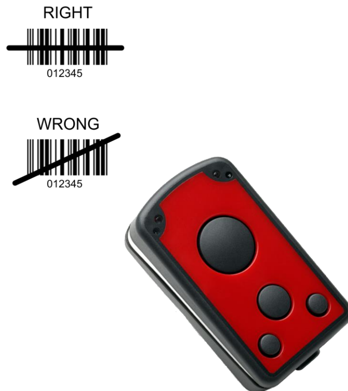
Fig. 2: Barcode Scanner Alignment
